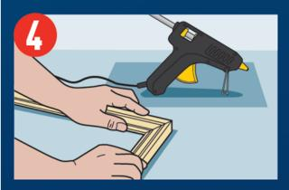
Immediately bring surfaces to be bonded together. Maximum bond strength developed after 2 minutes.
