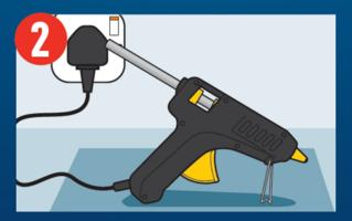
Place gun on stand on cardboard or wooden surface. Plug into mains. Leave gun to heat for 8-10 minutes.
