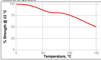
Cured for 5days @ 22°C Lap Shear Strength: Steel
