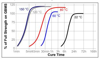
TYPICAL PROPERTIES OF CURED MATERIAL Cured for 7days @ 22°C, 1.2 mm thick samples. Physical Properties :
