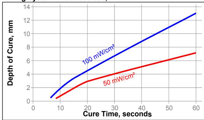
**Curing System: Electrodeless, H bulb**
