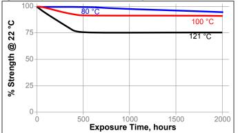
Aged under conditions indicated and tested at temperature
