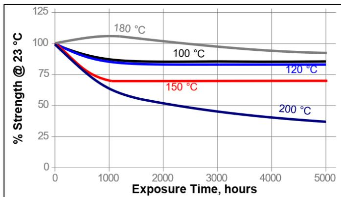
**熱老化/高温時強度**
